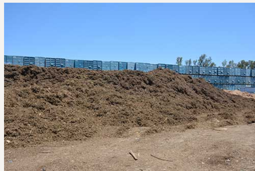
Organic waste is ground up before being fed into the Perris digester, which operates continuously to produce fuel and fertilizer.
