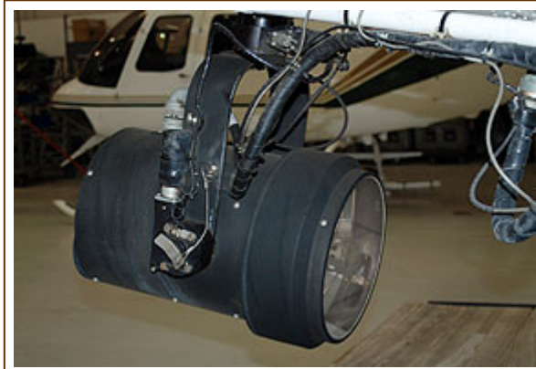
This 33-million candlepower searchlight can penetrate the best hiding places when law officers search for hidden suspects.
