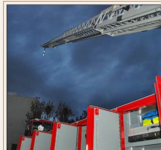
The Tiller comes equipped with a 100-foot extension ladder for high-rise firefighting.
