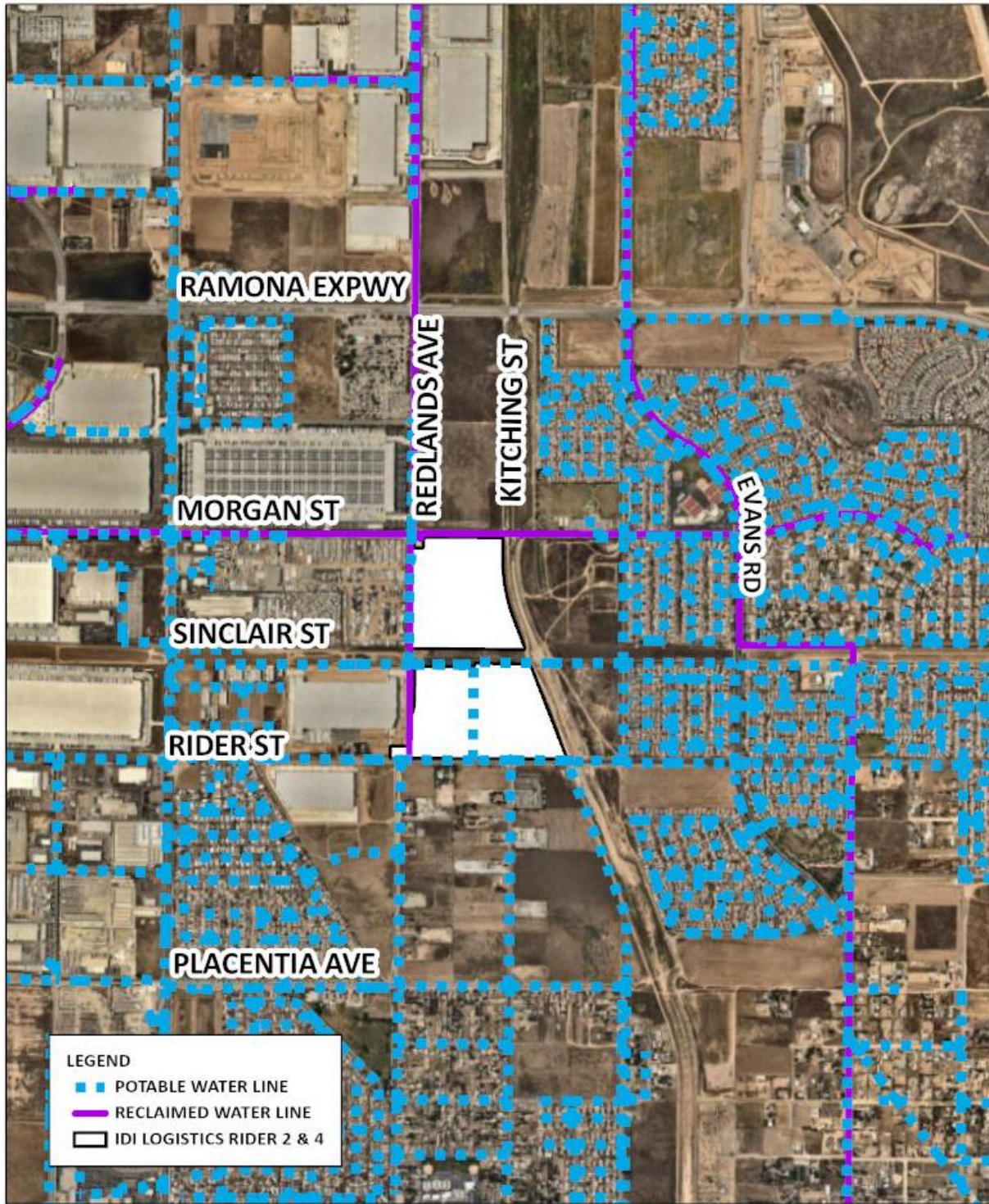
Figure 3: Project Location in Relation to Existing Waterlines
