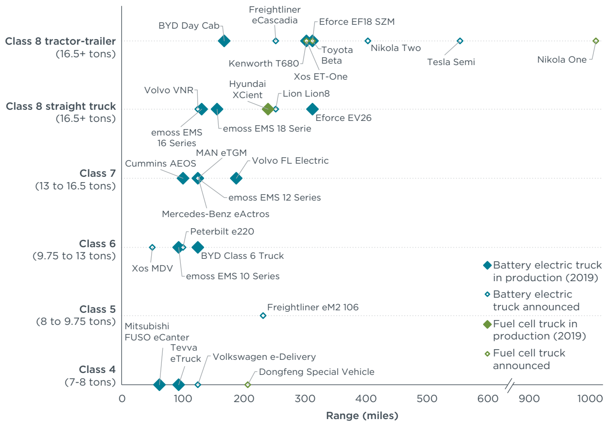
Figure 2. Range and GVWR class of announced or in-production zero-emission trucks
