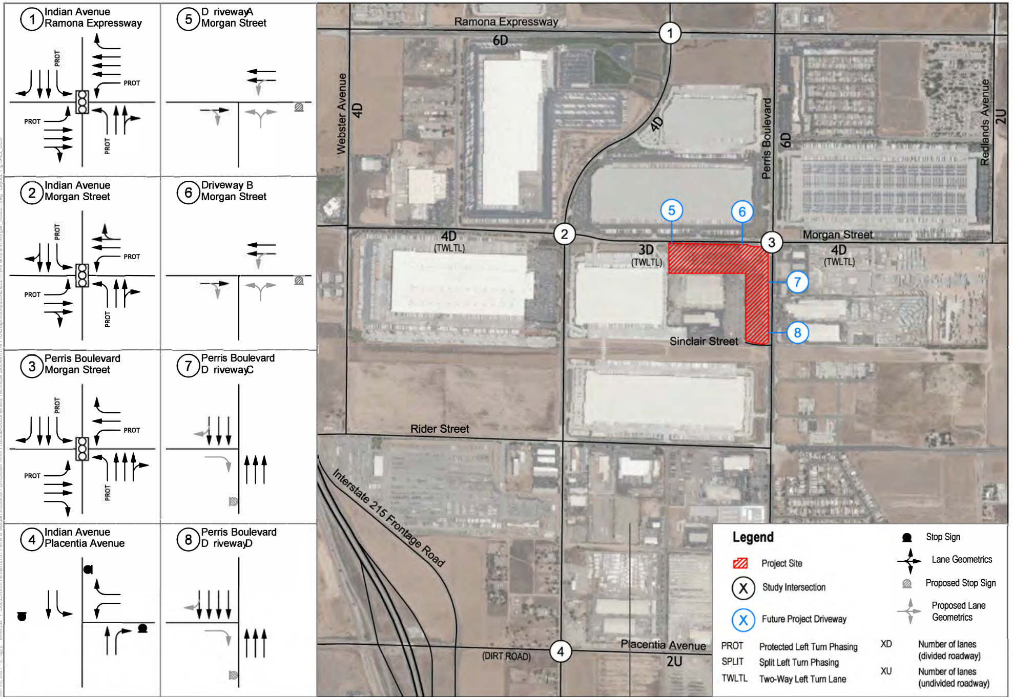
FIGURE 22 Existing Intersection Controls and Geometrics
