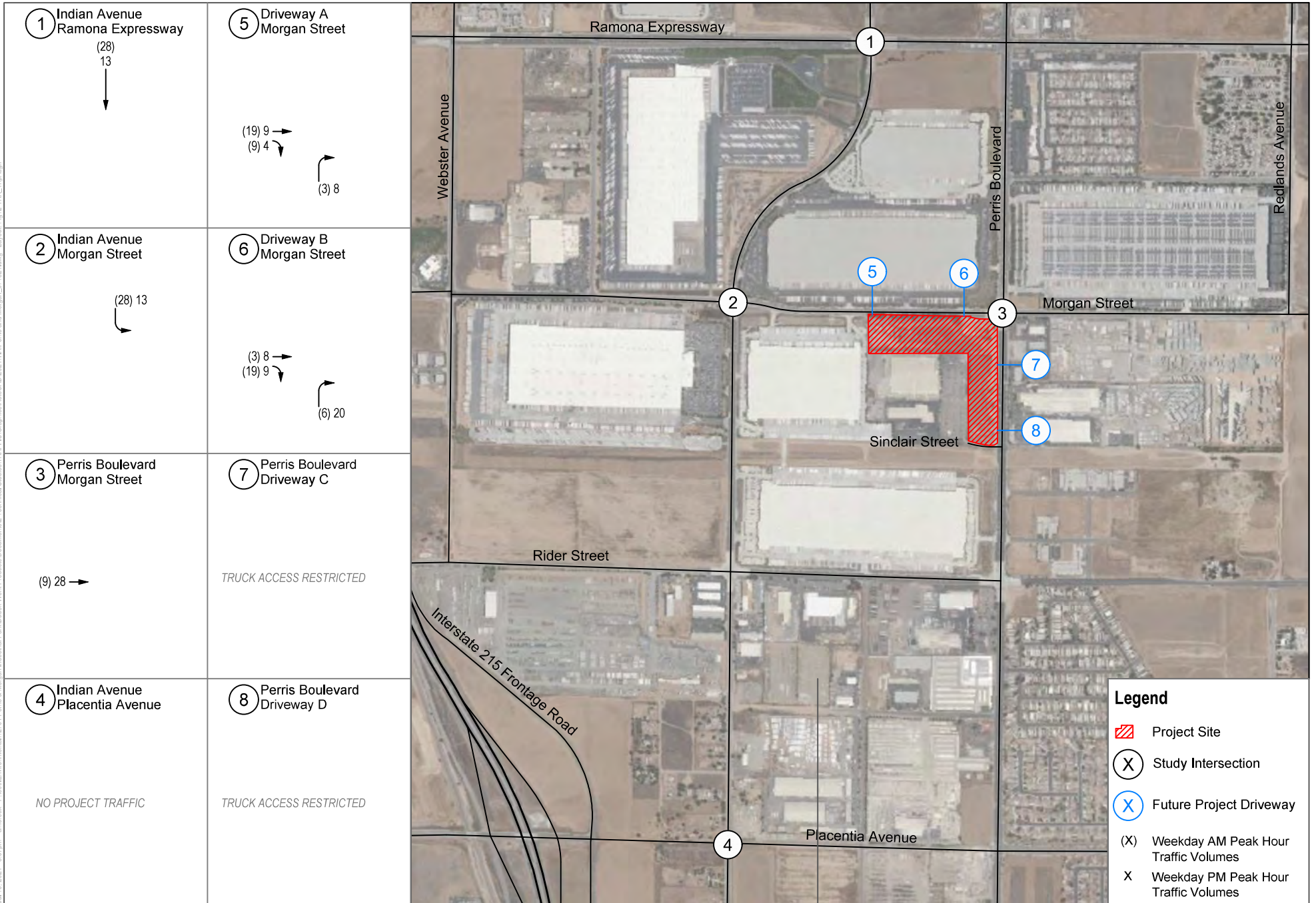
FIGURE 12 Project Truck Trip Assignment (PCE)
