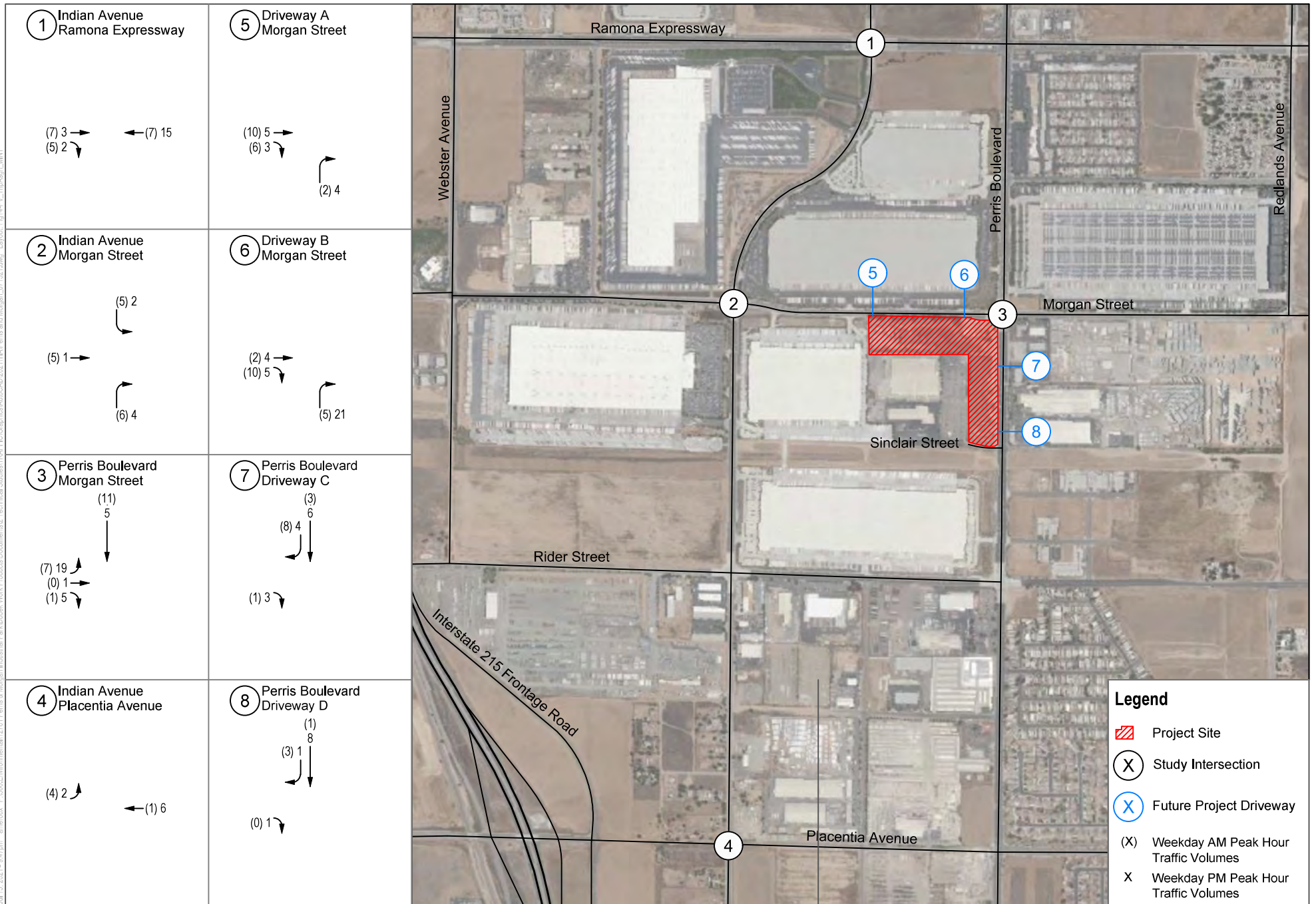
FIGURE 14 Project Passenger Vehicle Trip Assignment - With Placentia Interchange
