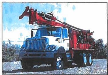
Figure 3. Mobile B-80 drill rig example.
