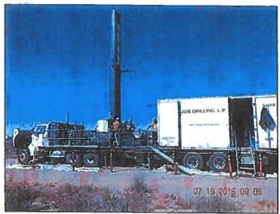
Figure 2. Sonic drill rig (white green, in left half of photo) with support truck (white box truck, on right side of photo).
