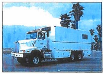
Figure 1. CPT drill rig example.
