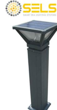
(c) SG9095 SOLAR BOLLARD LIGHT BY SELS. BOLT TO 18"Ø X 6" DEEP CONCRETE FOOTING WITH (4) 3/8" STAINLESS STEEL ANCHOR BOLTS PER MANUFACTURER'S RECOMMENDATIONS. COLOR TO BE BROWN. AVAILABLE FROM SMART ERA LIGHTING SYSTEMS 704-495-3535
