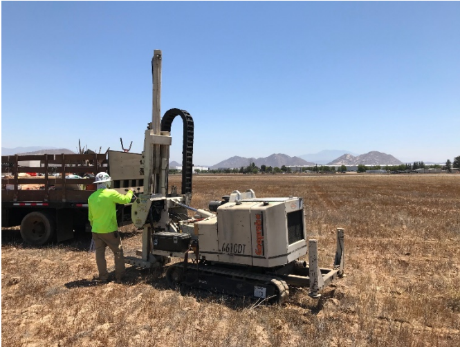
7. Geoprobe direct-push drilling rig set up at soil boring SB-5 in the northeastern portion of the Site
