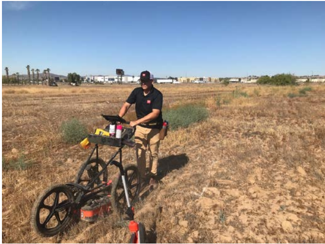
1. GPRS conducting utility locating and ground penetrating radar survey at SB-1
