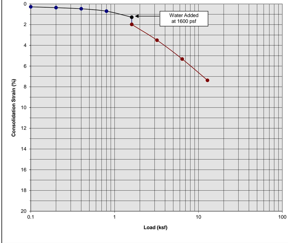
Classification: OLDER ALLUVIUM: Silty fine to medium Sand, trace Clay, trace coarse Sand
