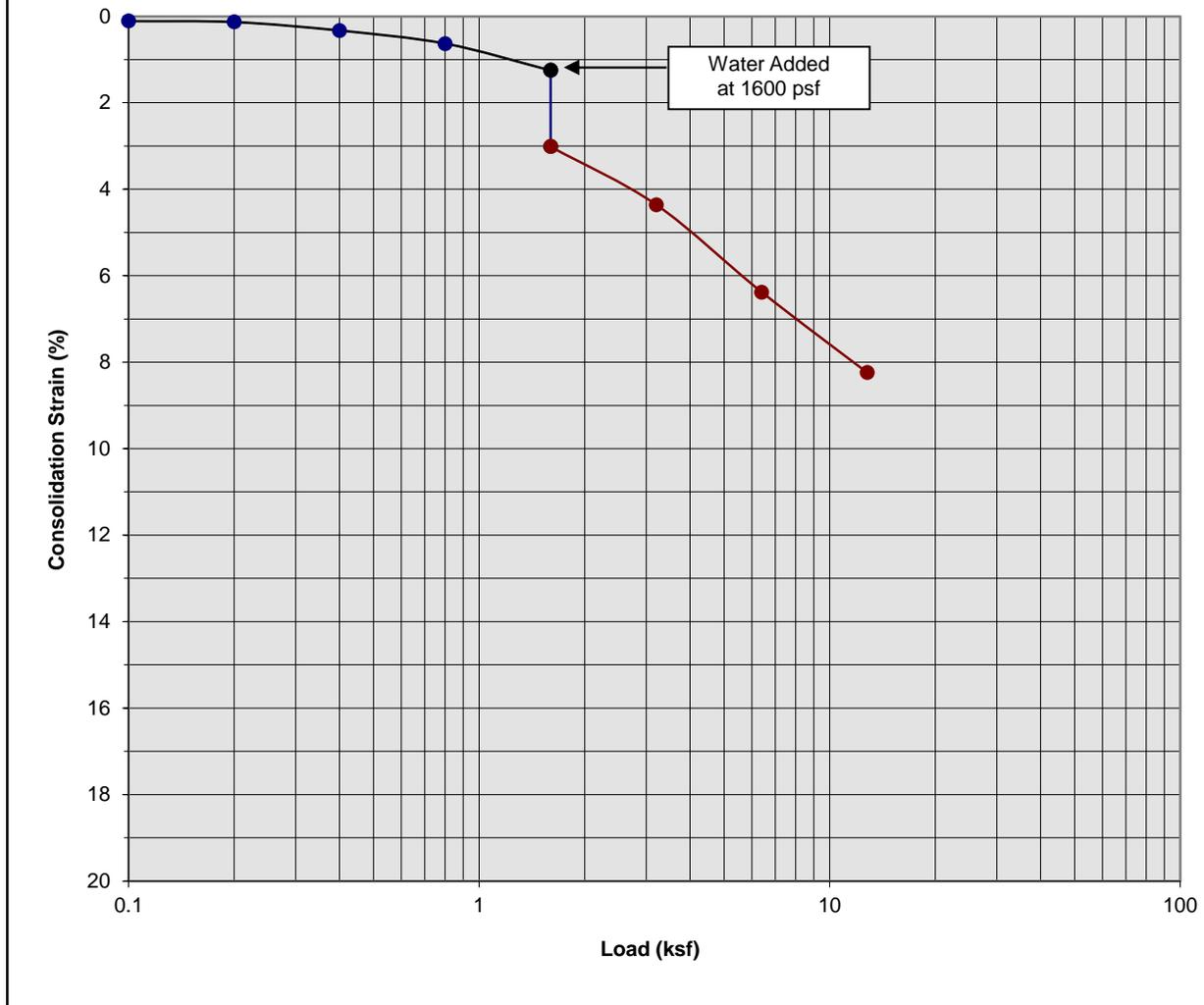
Classification: POSS. FILL: Silty fine to medium Sand, trace Clay, trace to little coarse Sand
