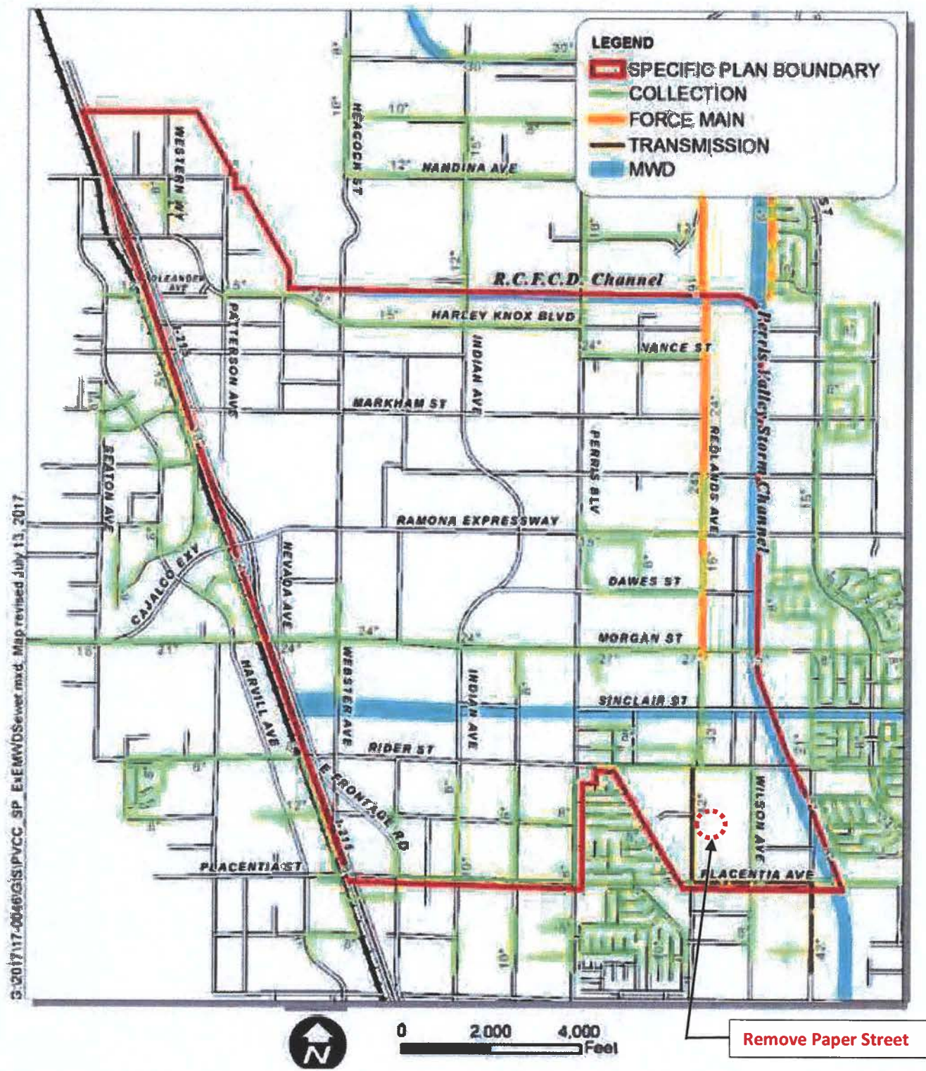
PROPOSED (Figure 3.0-8 Existing EMWD Sewer Map)
