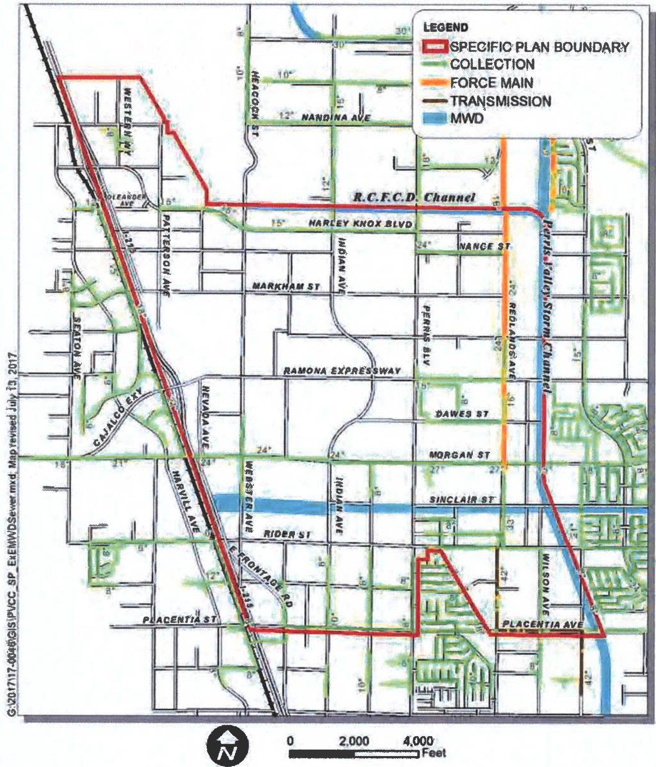
EXISTING (Figure 3.0-8 Existing EMWD Sewer Map)
