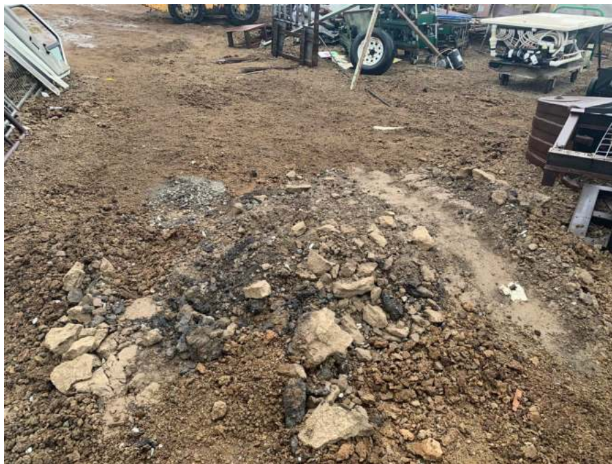
Photo #10 Eastern material storage area: asphalt mixed with soil.
