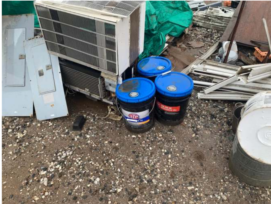
Photo #9 Eastern material storage area: 5-gallon buckets of hydraulic fluid located on bare soil.
