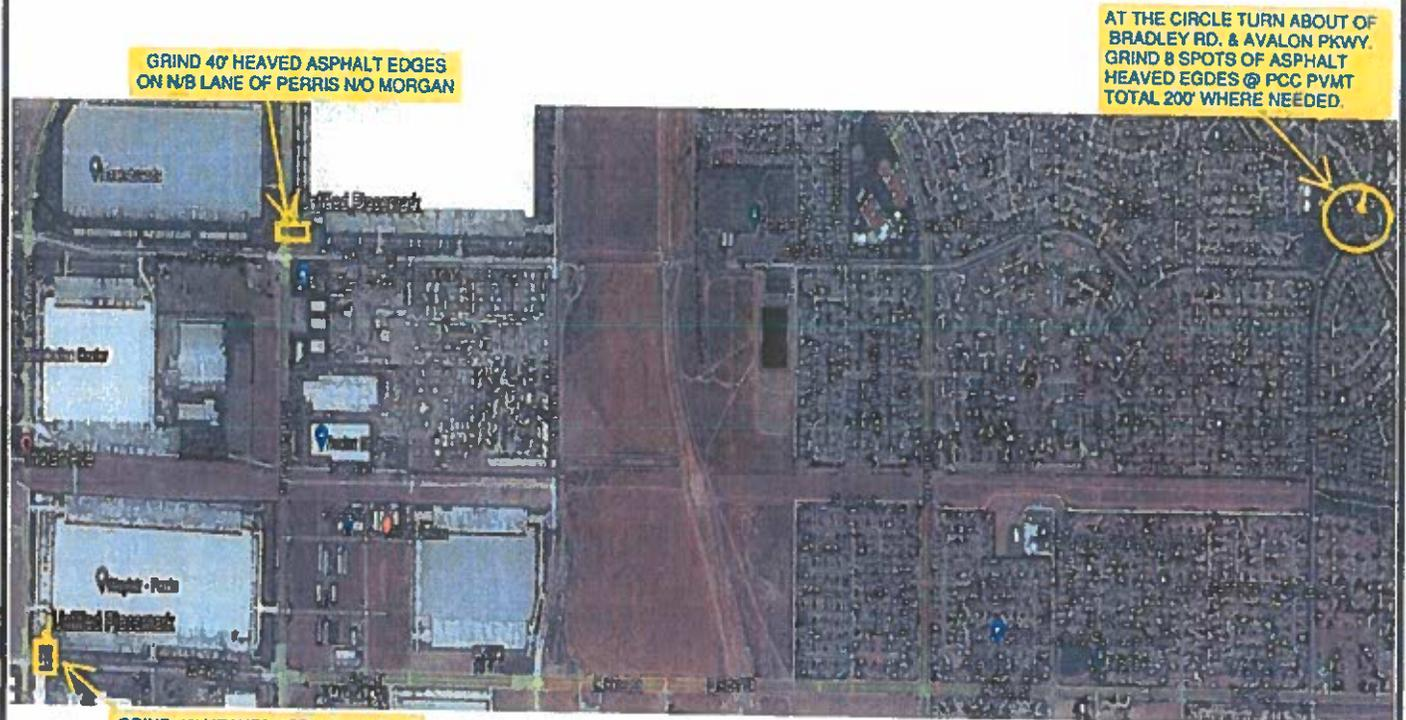
GRIND 40' HEAVED ASPHALT EDGES ON N/B LANE OF PERRIS N/O MORGAN
