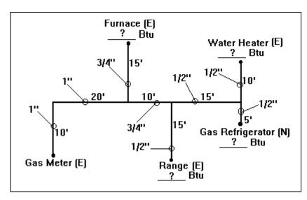
**NOTE: Section 1213.3 Test Pressure** New gas piping is required to be tested at a minimum of 10psi (69 kPa), for 15 minutes, with no pressure loss. The new gas piping must be under "pressure-test" at time of inspection.
