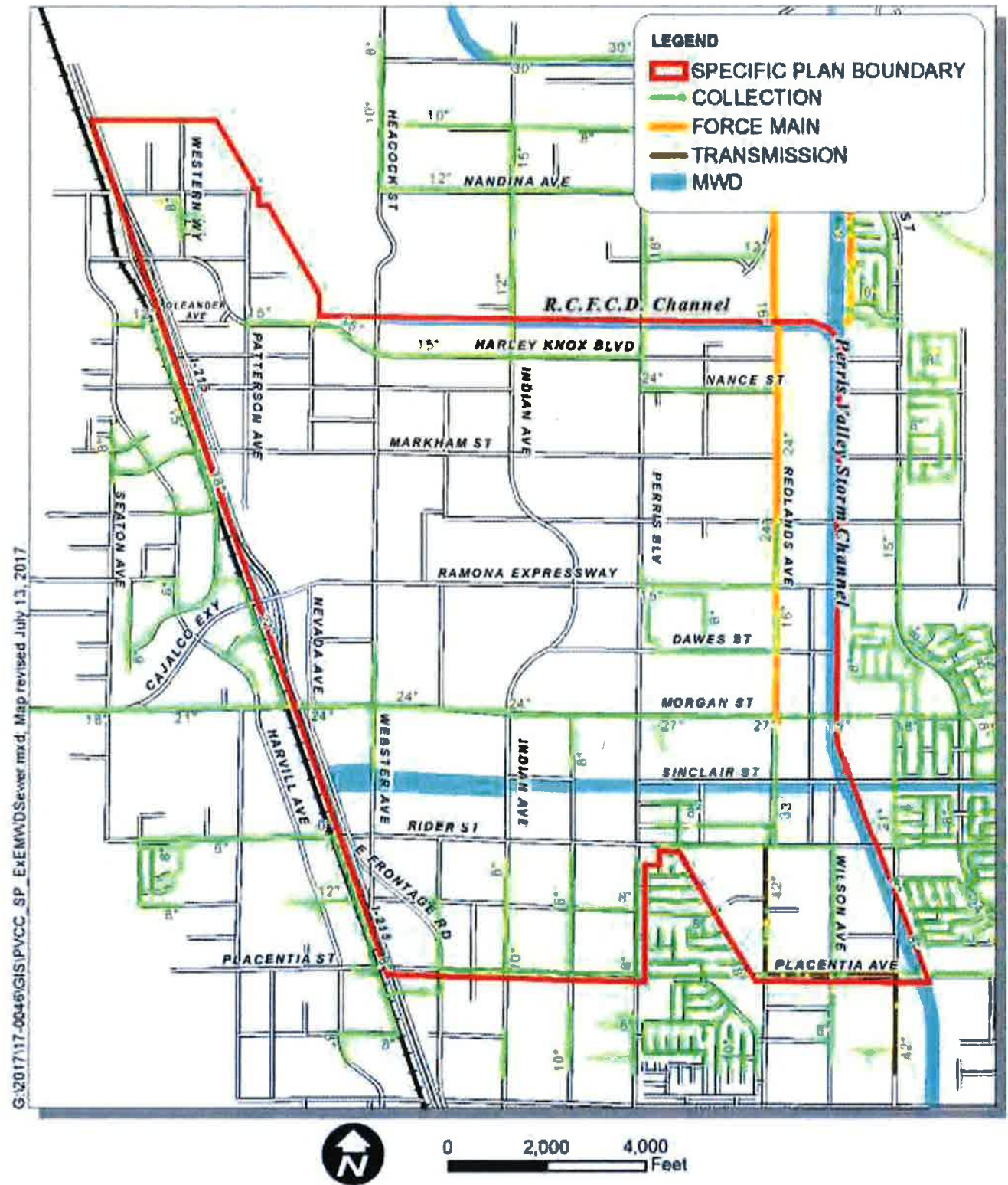
EXISTING (Figure 3.0-8 Existing EMWD Sewer Map)
