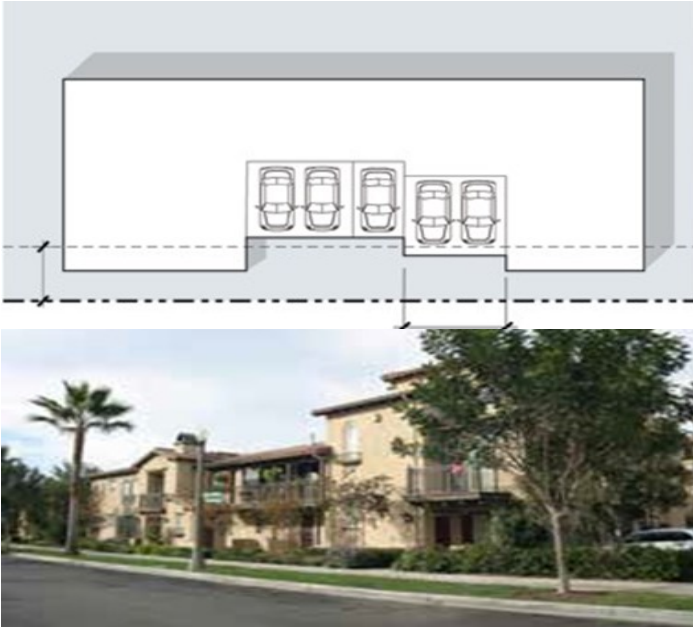
Standard 6.7.e: Garage doors should not be visible from the primary street. Where visible, garages should be recessed.
