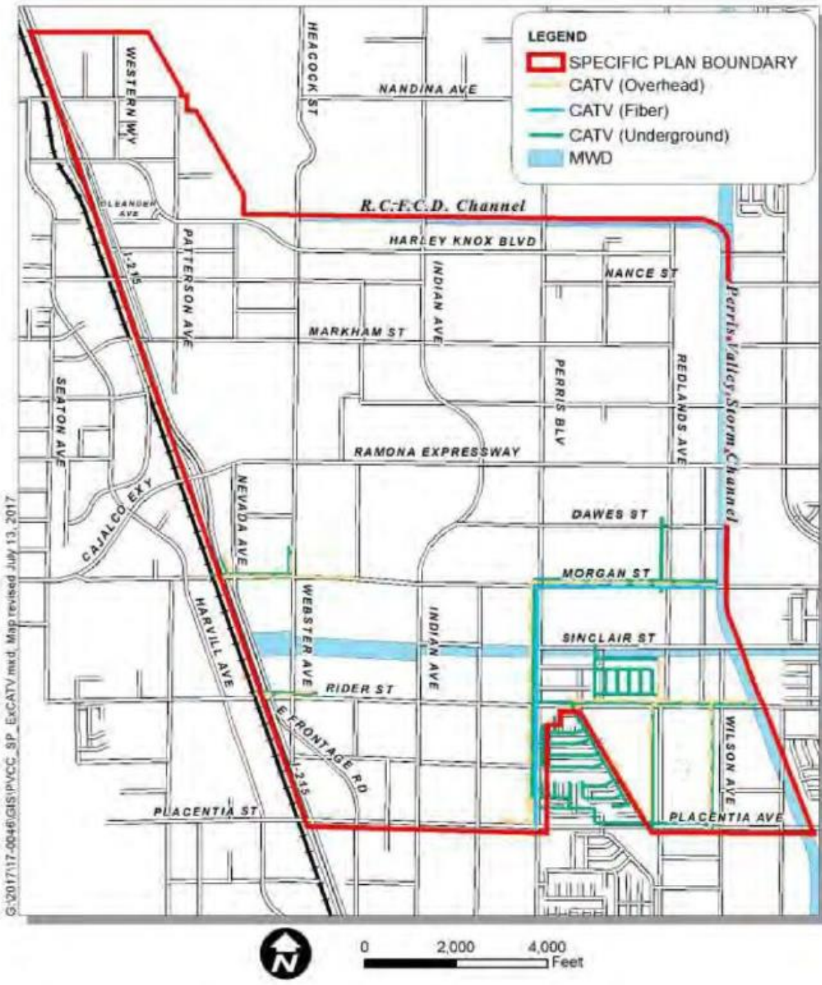
REVISED (Figure 3.0-15 Electrical Cable TV Map)
