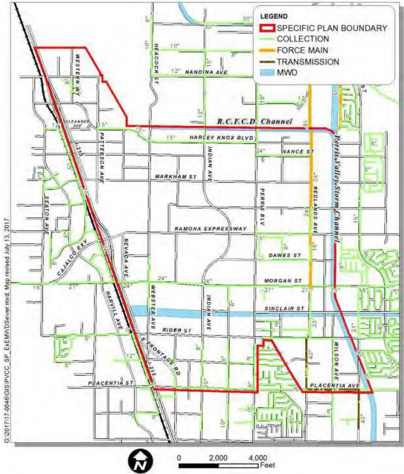
EXISTING (Figure 3.0-8 Existing EMWD Sewer Map)
