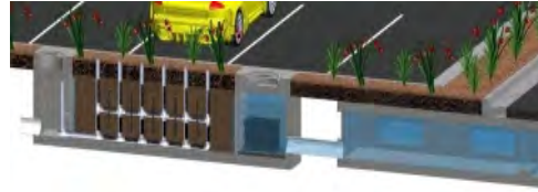
Horizontal Flow Biofiltration System
