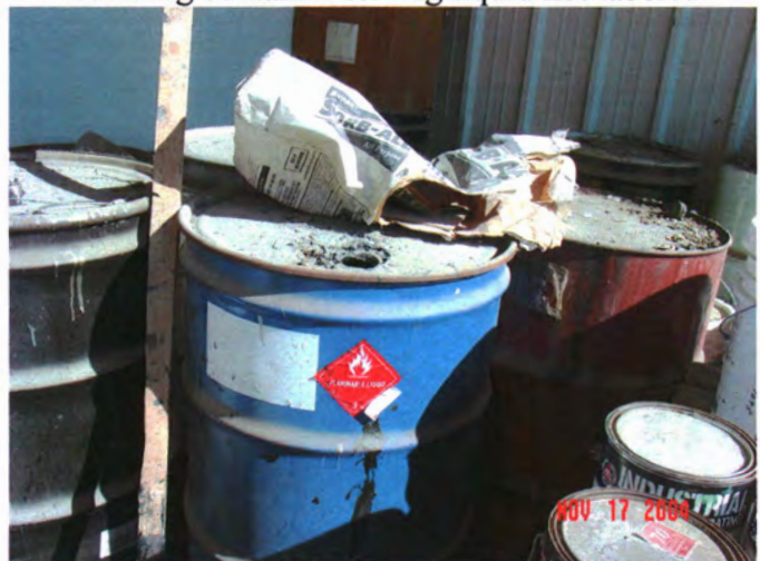
Open container in Haz Waste area/not labeled
