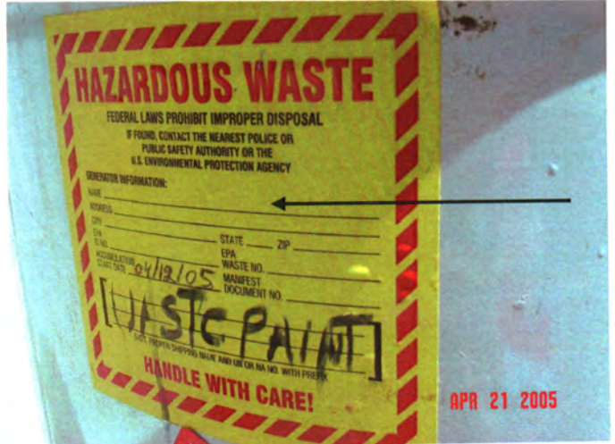
Haz Waste Label incomplete
