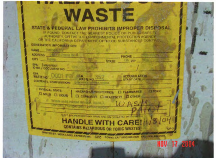
Improperly labeled Haz Waste date not properly placed
