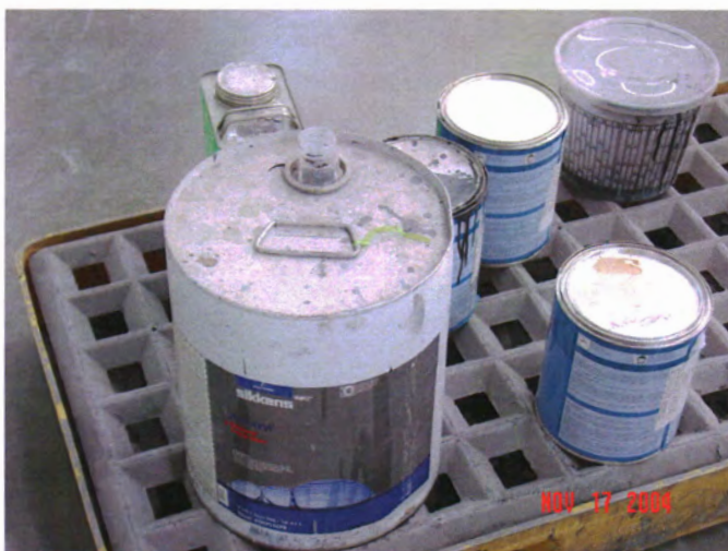
Open topped flammable liquid container
