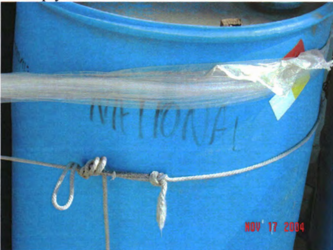
Drum labeled National is not proper labeling
