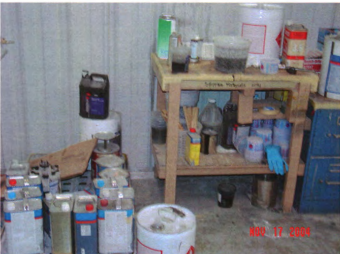
Open top containers with flammable liquid on self (two containers)
