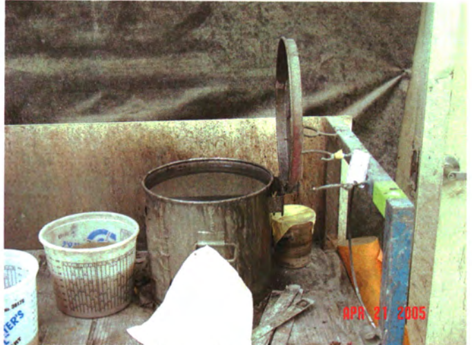
Open container with flammable waste
