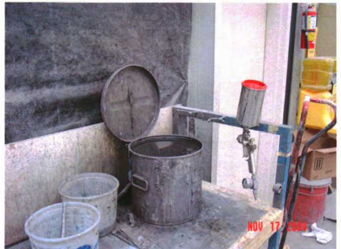
Open container with flammable liquid
