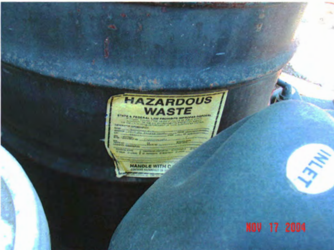
Used oil stored in plastic drum no label - empty drum labeled Haz Waste
