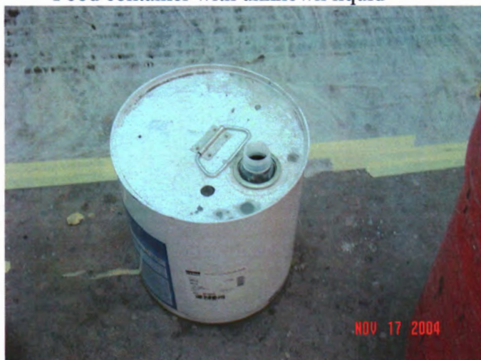
Open container of flammable liquid
