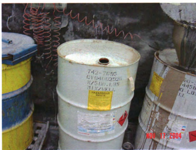
Open waste paint drum not grounded was drum not labeled
