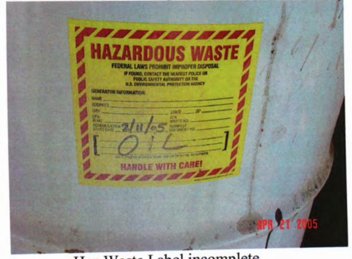
Haz Waste Label incomplete
