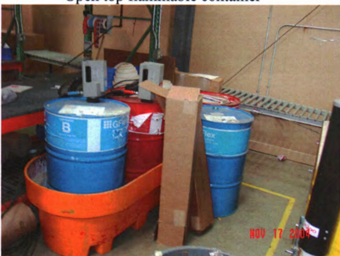
Open top flammable container
