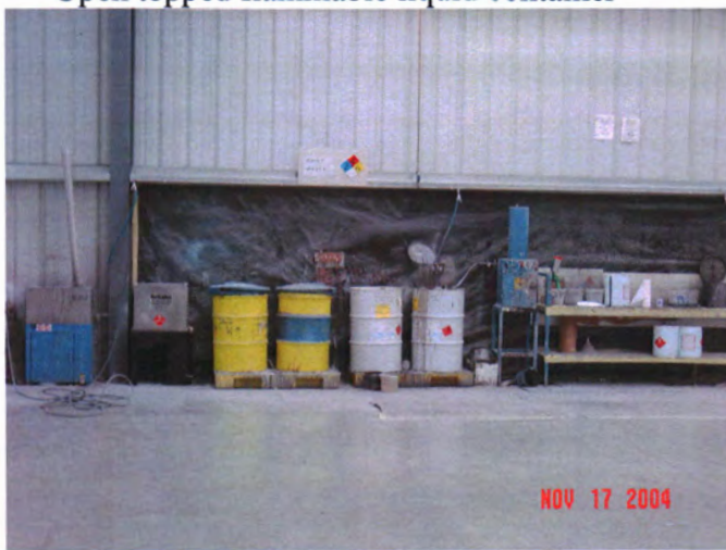
Open topped flammable liquid container
