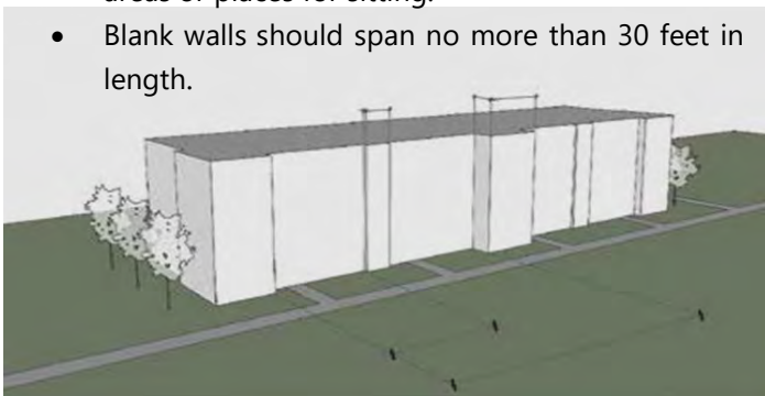
Standard 6.3.a and Standard 6.3.b: Multi units building should have Major and minor massing breaks to reduce bulkiness.
