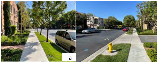
Standard 2.5.c. An 18-inch concrete strip should be provided next to the end parking stall.
