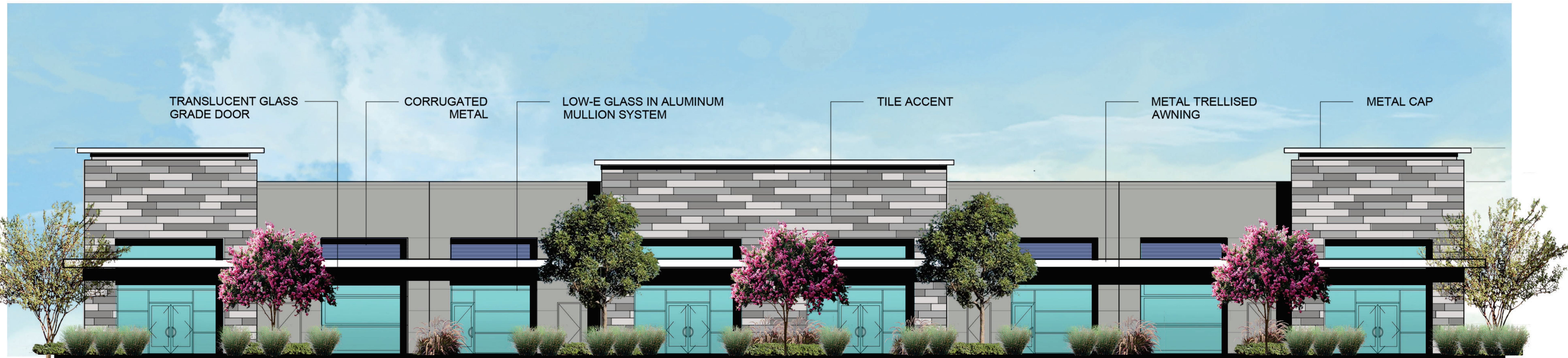
BUILDING 2 EAST (TRUMBLE ROAD) ELEVATION
