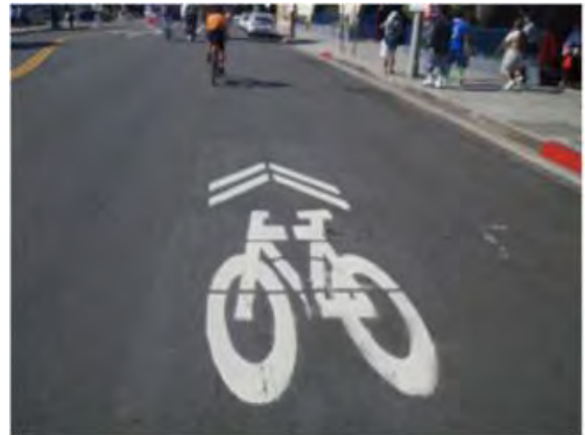
Class III Bike Route with Sharrow Stencil
